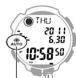
Auto light switch on indicator
