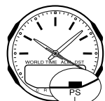
Power Saving indicator
